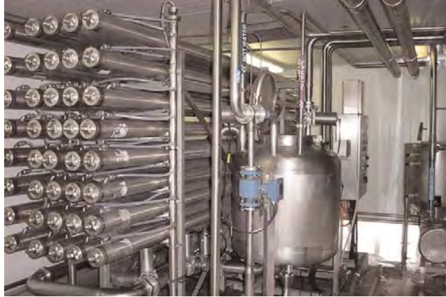
Membrane processes have provided the dairy processing industry with the means to produce value-added by-products that were previously sent to waste or used as stockfeed.
