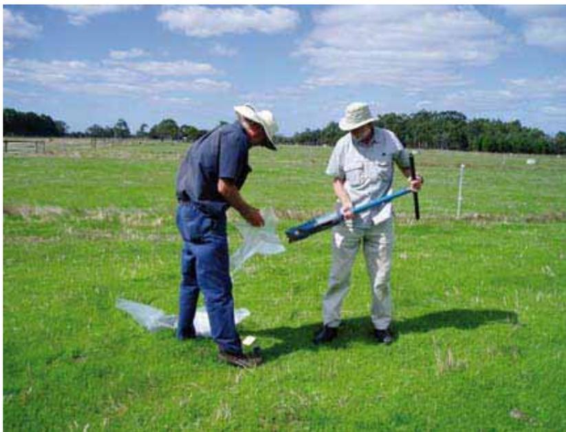
Figure 3.1 Soil sampling using an auger
