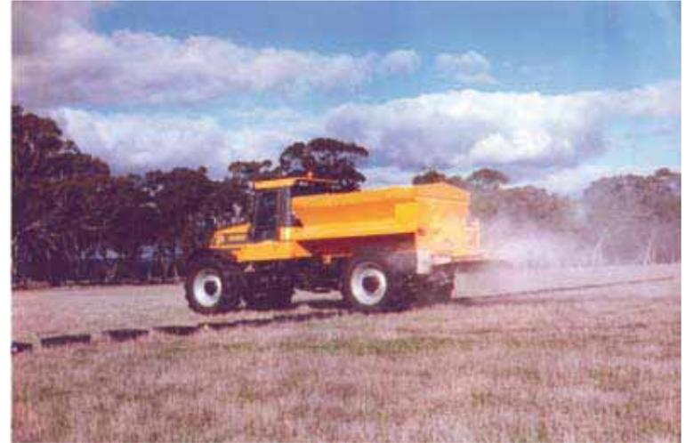
***Most fertilisers are corrosive to steel.
