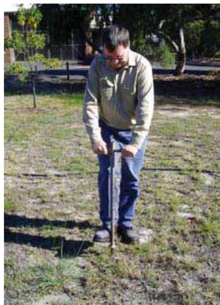
Figure 3.2 A sampling pogo is a metal tube about 2.5 cm in diameter that is pushed into the soil to a depth of 10 cm.
